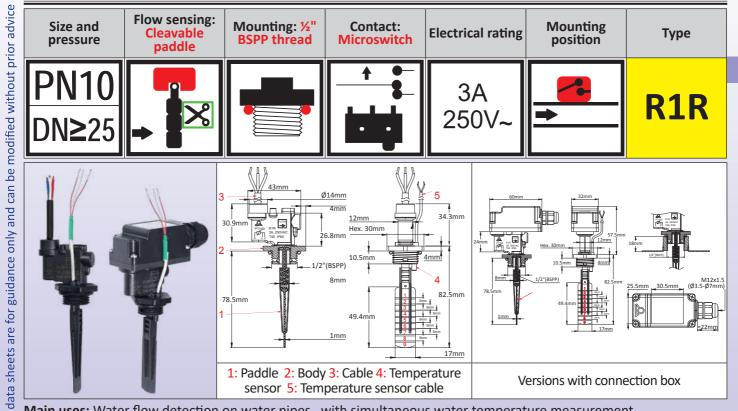
Main uses: Water flow detection on water pipes, with simultaneous water temperature measurement Functional principle: Balanced paddle, perpendicular to the main flow, actuating a micro-switch. Flexible elastomeric gasket between paddle and electric switch. Temperature measurement is made by a plastic pocket located under the 1/2" thread
