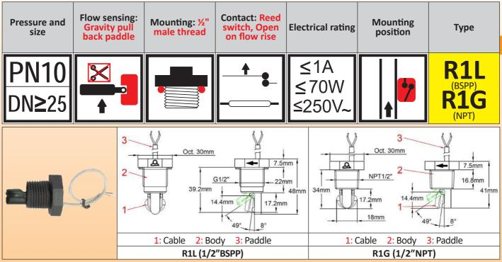
**Main uses:** The most simple and price effective flow switch of the range. Used for water flow detection on **small size** water pipes. **CONTACT OPENS BY FLOW RISE.**
