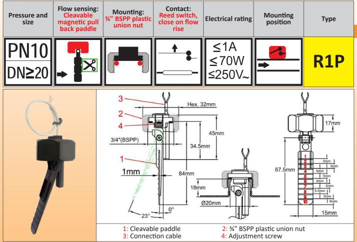
Main uses: The most simple flow switch with magnetic pull-back. Recommended mounting position is on horizontal pipes, but can be mounted in any position. For water flow detection on dia 25 to 100mm water pipes **Functional principle:**
