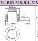
1/2" BSPP female fitting, 304L stainless steel, for welding on 27.6mm hole
