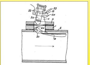
In 1931, the first paddle switch with a magnetic action is invented by Louis E. Richmond (US Patent 1888737). A paddle with a metallic roller actuates a balanced magnet with a mercury switch located outside.
