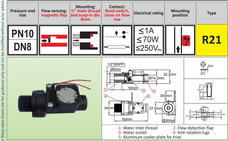
Main applications: Product developed for miniature instantaneous water heaters for showers. The mobile flap system provides compactness. Water inlet is done directly by the ½" BSPP male thread. Mandatory vertical mounting, with water inlet from the bottom. Connection to internal copper piping DN8 and DN10 with quick coupling. A built in aluminum heat exchanger, in contact with the cold water input is provided to cool a triac.
