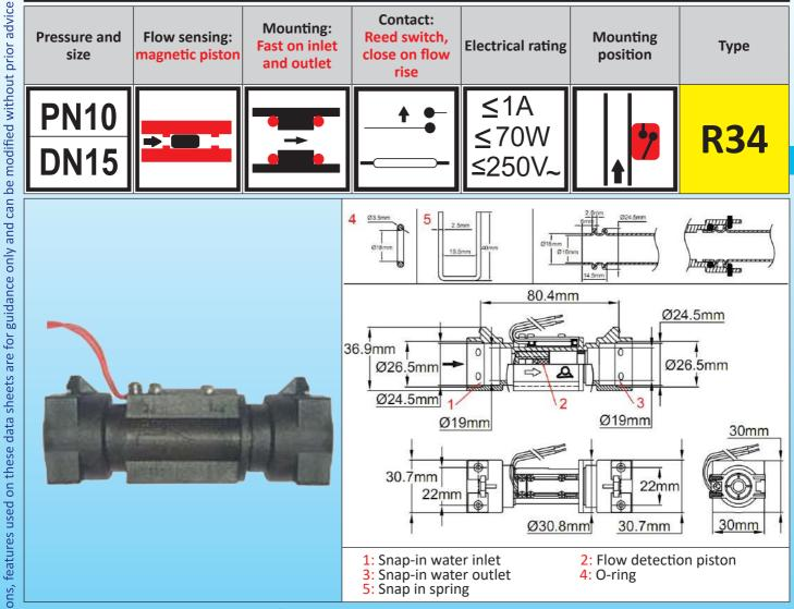
Main applications: Product developed for electrical or gas instantaneous water heaters. Snap in water inlet and outlet for copper tubes. Mandatory vertical mounting, with water inlet from the bottom.
