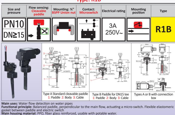
Main housing material: PPO, fiber glass reinforced, usable with potable water. Paddle material: Polypropylene, resistant to ozone and water disinfection products Paddle gasket: Santoprene, resistant to ozone and water disinfection products
