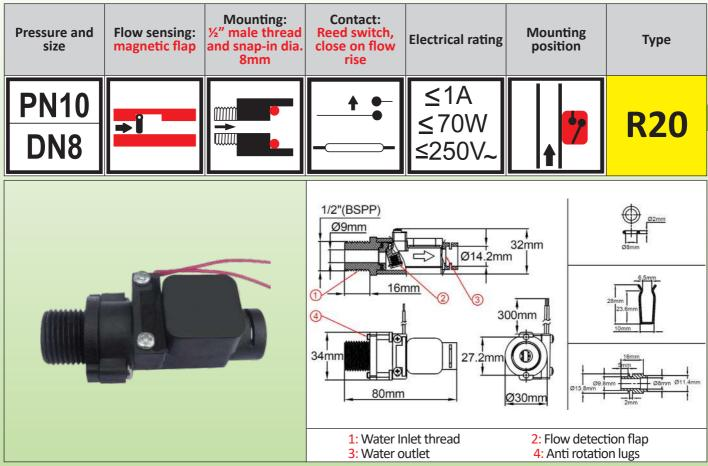
**Main applications:** Product developed for miniature instantaneous water heaters for showers. The mobile flap system provides compactness. Water inlet is done directly by the ½" BSPP male thread. Mandatory vertical mounting, with water inlet from the bottom. Connection to internal copper piping DN8 and DN10 with quick coupling
