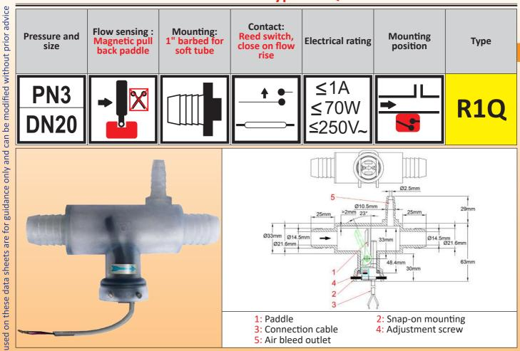
Main uses: Tee equipped with paddle flow switch, for spas and swimming pools applications, mounting on 1" (20 to 21mm ID) soft PVC tubes, adjustable setting.
