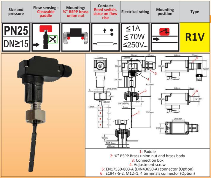
Main uses: General application in flow detection. Recommended mounting position is on horizontal pipes, but can be mounted in any position. For liquids flow detection on dia. 15 to 100mm pipes. Body and union nut in brass for improved mechanical strength and pressure resistance. Connection box with terminal block or connectors, and detection point adjustment screw
